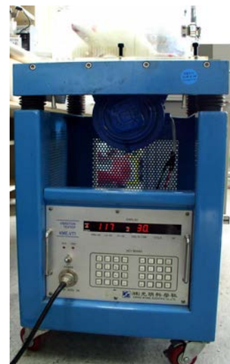
Figure 1. Vibration test machine to whole body of rats.
